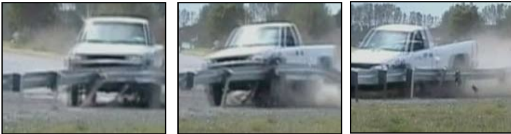
Test Level 3 crash test of NU-GUARD-27 design.
