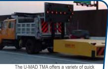
The U-MAD TMA offers a variety of quick mounting options to make deployment and removal safe and easy.
