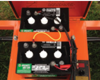
Front of box folds down to allow for easy removal of the batteries
